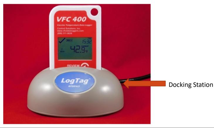
•Now that we have made sure our data logger is in the docking station we can return to the profile manger we left open.
